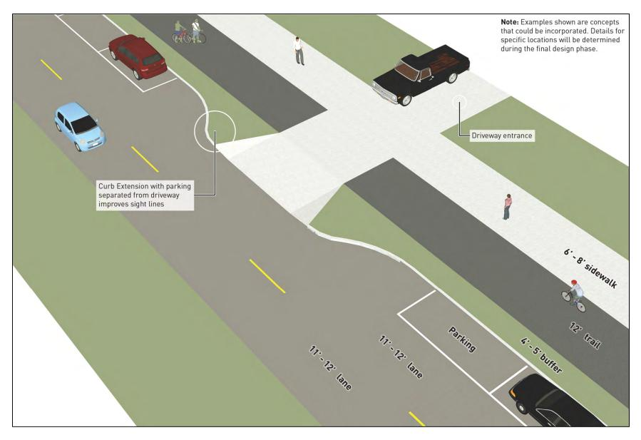
Figure 1-9. Intersection Design Options: Curb Extension
