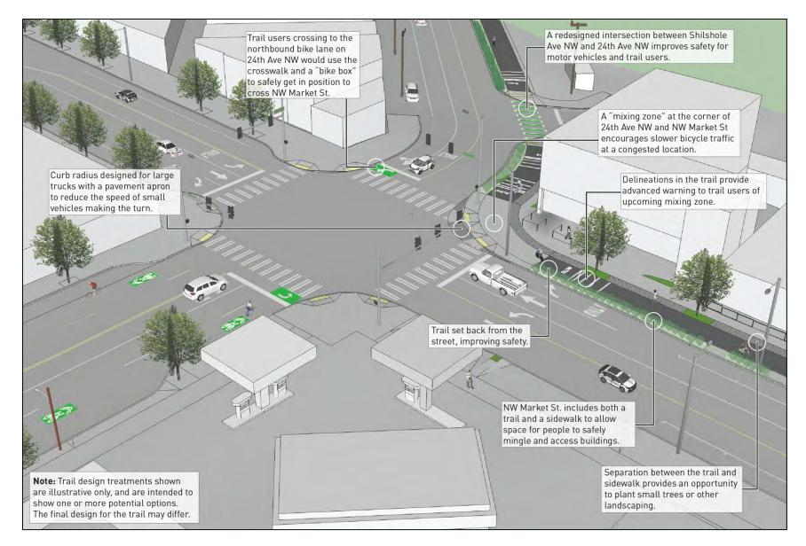
Figure 1-5. Potential Roadway Design and Safety Modifications (NW Market St and 24<sup>th</sup> Ave NW)
