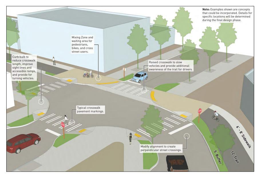
Figure 1-10. Intersection Design Options: Raised Crosswalk
