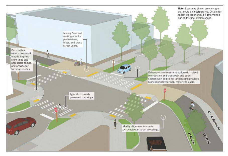
Figure 1-11. Intersection Design Options: Driveway Style Intersection
