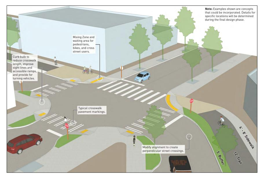
Figure 1-7. Intersection Design Options: Perpendicular Intersection
